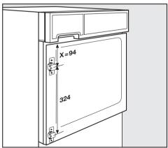
Mark the two hinge holes and the four smaller holes as shown in the diagram.
